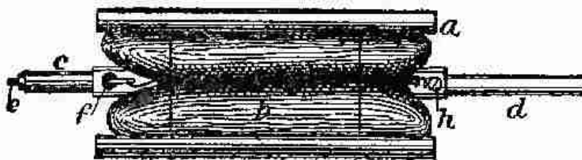
Armature of Generator.
