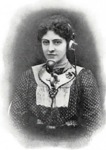
Breastplate Transmitter, and Headgear Receiver as used in conjunction with one another.
