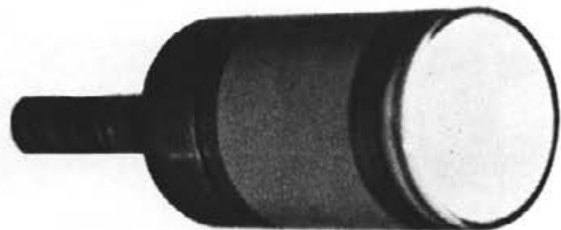
73 Seven-inch Charactron shaped beam tube.
