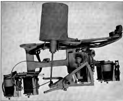
FIG. 47.—Unmounted master switch.
