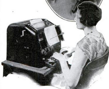
Teletypewriter Machines and Switchboard Making Possible a Two-Way Message Service between Subscribers
